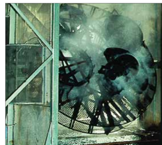
ROMOLD rotational moulding production (water cooling)
