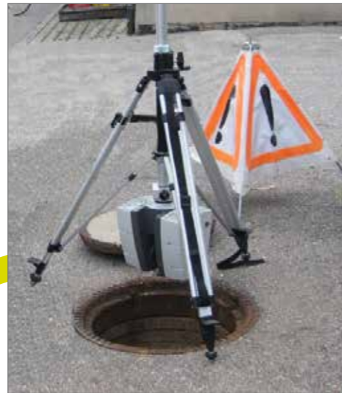
Detailed chamber measurements ideally via chamber scan
