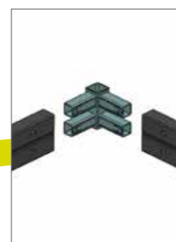
vertically separable, profile with corner connecting elements, drainage opening in base plate
